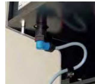
Standard power/signal connector Most Ekta™ lights use similar 7-pole receptacle.
