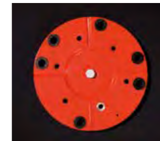
Installation The bottom plate supports installation on structure with 3 x M12 bolts on a 200 mm diameter. The mounting holes are galvanic isolated with plastic isolators. PTFE breathing vent for pressure release.
