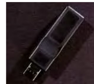
Programming with PC Using Sabik USB interface.
