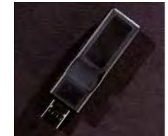
Programming with PC Using Sabik USB interface.
