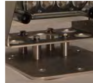
Pedestal Combination of three and four \text{Ø}16 mm mounting holes on a 200 mm ring. Horizontal beam alignment within \pm 8^\circ is possible by turning the light unit on the pedestal.
