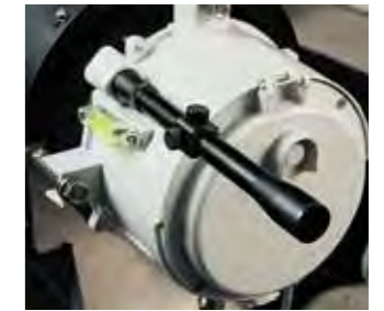
Precision alignment A gun sight can be used for precision alignment to the center line of the range.
