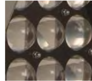
High power LEDs and custom optics Flexible platform for several horizontal divergence alternatives.
