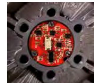
OFBS The Optical Feedback System (OFBS) enables built-in monitoring of LED degradation over time.
