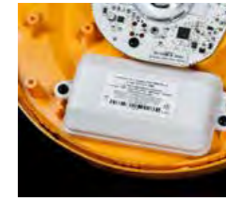
Li-ion Replaceable Li-ion battery pack with extreme temperature range and up to 8-year life expectancy.
