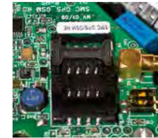
Remote monitoring GSM unit and antenna integrated in the lantern for remote monitoring and control. For more information, please see the LightGuard Section.
