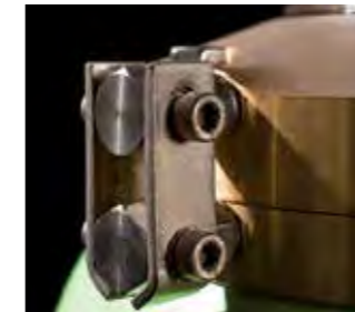
Hinged The primary battery can be changed easily as hinged flanges allow the lantern to open safely in sea conditions. The lantern acts as the waterproof door to the battery cabin.
