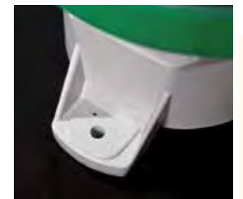
Installation Supports installation on structure using 3 x M6 bolts on a 150 mm diameter.
