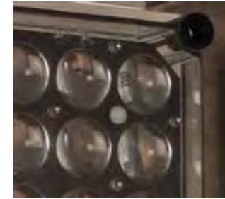
Integrated light sensors Redundant leading light systems may use either integrated or additional light sensors.
