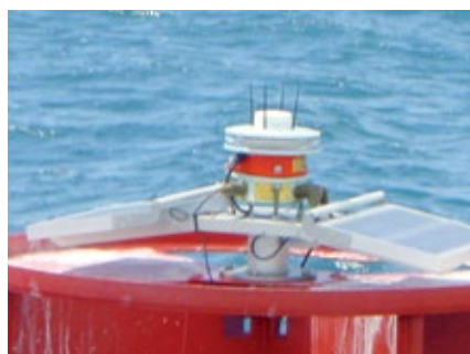
The VSU-29 mounting option for a Vega VLB-44 beacon includes the mounting ring.
