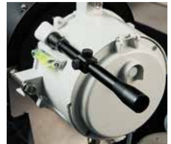
Precision alignment A gun sight can be used for precision alignment to the center line of the range.
