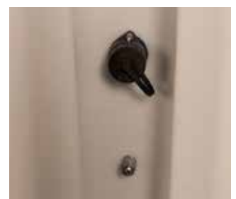
Auxiliary connector Enables external charging or additional solar module.
