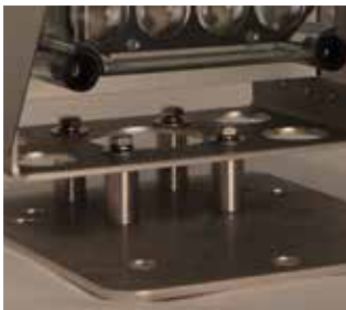
Pedestal Combination of three and four \text{\O}16 mm mounting holes on a 200 mm ring. Horizontal beam alignment within \pm 8^\circ is possible by turning the light unit on the pedestal.
