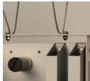
Sighting Scope mount Mechanical interface for attaching an optional Sighting Scope.
